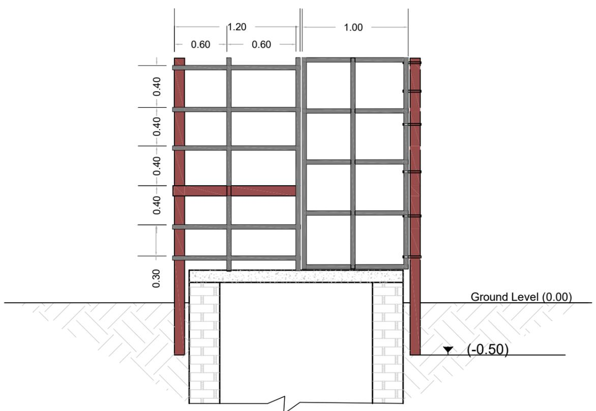
Typical section of super structure at (2-2)
