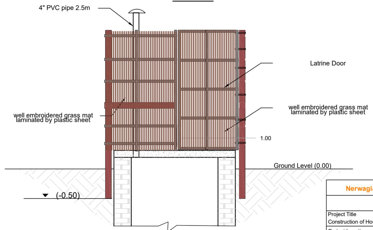
Typical section of super structure detail
